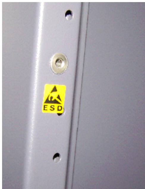
Figure 1-53 ESD jack of the N66E-22 cabinet
