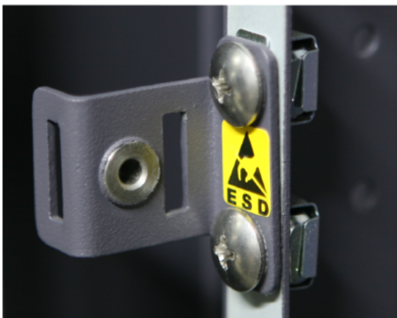
Figure 1-11 ESD jack of the N63E-22 cabinet
