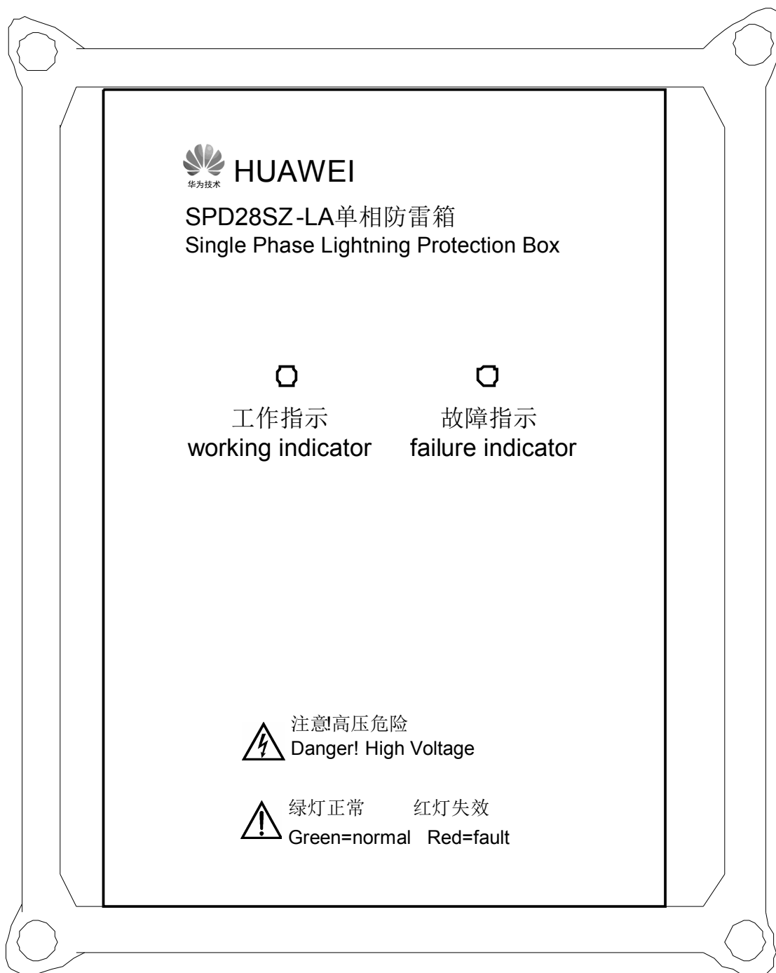
Figure 6-17 Front panel of the SPD28SZ surge protector
