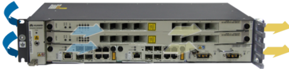
Figure 2-33 Ventilation of the MA5608T chassis
